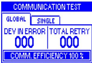
Number of sensors on which communication errors occurred (**DEV IN ERROR**) and total number of transmissions repeated against detected errors (**TOTAL RETRY**). A maximum of 5 transmissions are repeated for each sensor.
