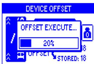
The **OFFSET EXECUTE** bar indicates the offset operation in progress (percentage of calibrated sensors).
