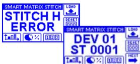
High tension error (*the tension detected by the sensor 01 is out of the threshold and/or time limits set up in **TENS HIGH** and/or **HIGH TIME** parameters*).
