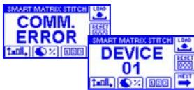
Communication error between SMART MATRIX STITCH terminal and sensor 01.
