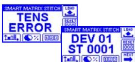
Tension error detected during the stand-by period and/or during the stitching execution (*see examples on chapter “Style Programming” **STYLE EDIT***) - ADV window
