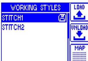
"**LOAD STITCH STYLE**" appears for a few seconds and then the display turns back to the **LOAD** menu, with the new style loaded.
