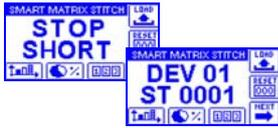
Short circuit or overload on the TS55 sensor STOP output
