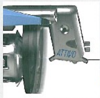
ATMO (optional) keeps constant tension, electronically driven
